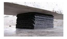
Scrap rubber tire can also used for the base isolation. There are very large amount of friction between the two tire pads so it can be stick two tire together. Although there may be some slip between he tire, that would also helpful in the dissipation of energy. Rectangular shaped layers cut from tread sections of used tires and then piled on the top of each other to form scrap tire pad can function as an elastomeric pad.
