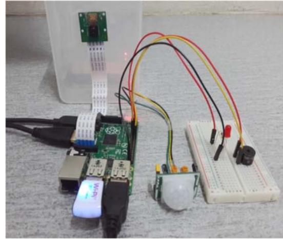
Fig.4. Motion detecting camera security system experimental setup
