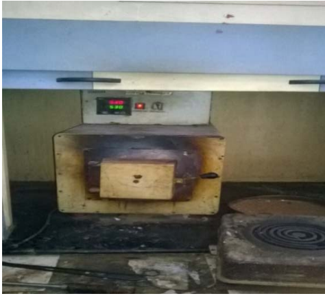
Fig 3: Solutionizing of Composite at 530°C
