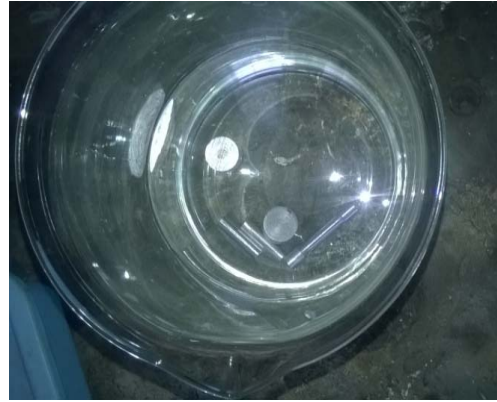
Fig 7: Aqueous polymer Solution (PEG) quenched Specimens
