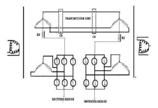
Fig.1.Basic Circuit of AC-DC transmission
