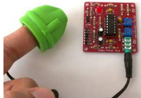
Figure 5: PC connected heart beat sensor
