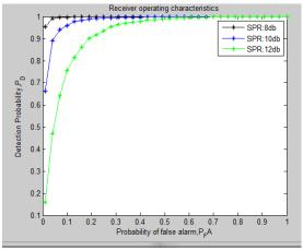
Fig 9.2 Receiver operating characteristics
