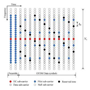
Fig 1.Time-frequency allocation for one OFDM frame [1]
