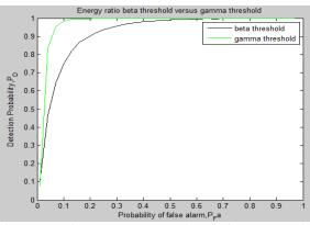
Fig 9.5 Performance comparison of energy ratio and modified energy ratio algorithms
