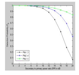
Fig 9.3 Detection probability versus SPR
