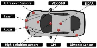
Figure 4. Key technologies enabling autonomous cars.
