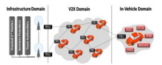
Figure 1. ITS high level architecture. RSU, road side unit; OBU, on-board unit; AU, application unit; ECU, electronic control unit; TPM, trusted platform module. Finally, a Global Navigation Satellite System (GNSS) unit is used to obtain accurate location information. The V2X domain (or ad hoc domain) consists of vehicle OBUs and roadside units (RSUs) deployed along the roads. As shown in Figure 1.
