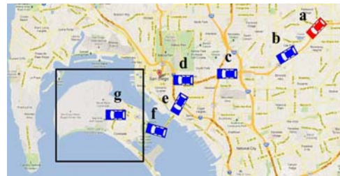
Fig 3. Geographical location based encryption, the only node (g) in the shaded region can only decrypt and access cipher text sent by vehicle (a).
