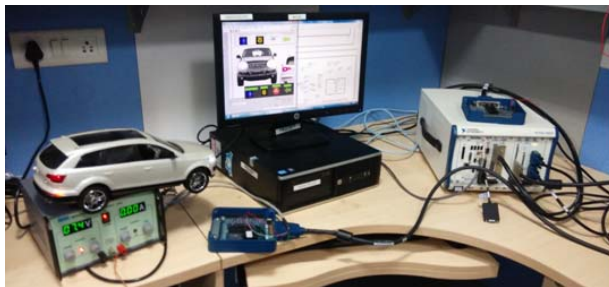
Image. 2:-LABVIEW HIL setup Demonstration
