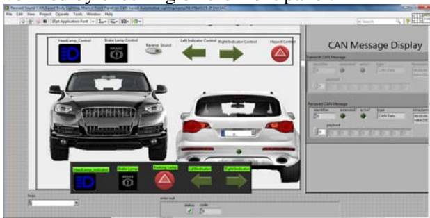
Image. 3:- Output of CAN communication on LABVIEW
