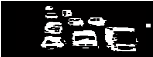
Fig 4: Moving vehicles detection using background subtraction method
