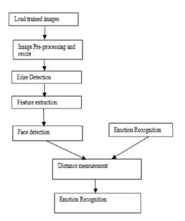
Fig 2.Functional block diagram of the facial recognition system.
