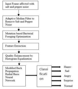
Fig11. Block Diagram of Hybrid Technique
