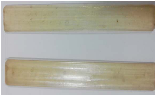
Figure 3.3: Photograph of Polyester-E-Glass composite specimen
