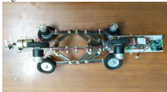
Fig.17 – Fully assembled pipe inspection robot Working: The complete assembly of the robot leads to the next phase of the project – Working. Here the robot is checked for its performance of
