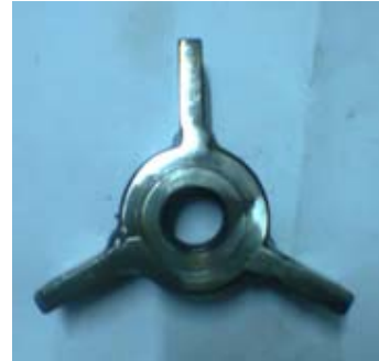
Fig. 11 – Welding of Nut strips
