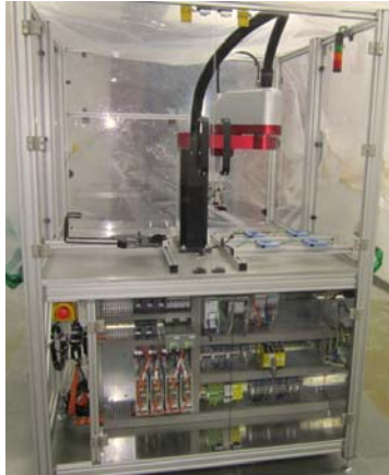
Figure.6. Robotic Trainer kit There are two drives contains a Software CD, Ethernet cable & Power cables. In this kits, participants can do demo experiments. Photo of Drive.
