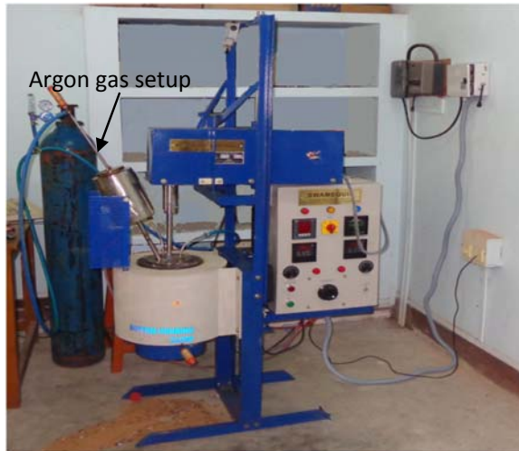
Fig. 1 Experimental setup used for the fabrication of nanocomposite
