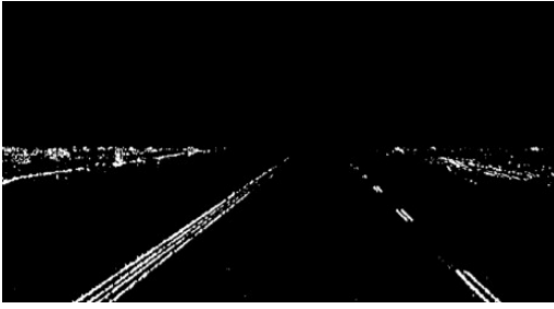
Figure 3.3 image with detected edge pixel
