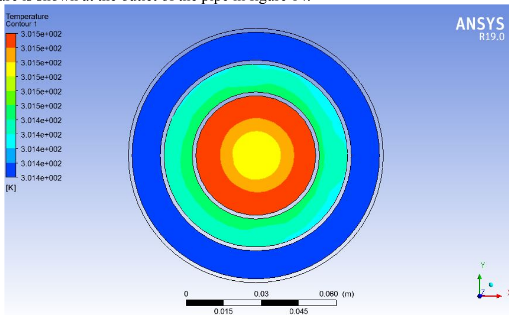
Figure 14: Temperature at outlet of pipe with 25% porosity
