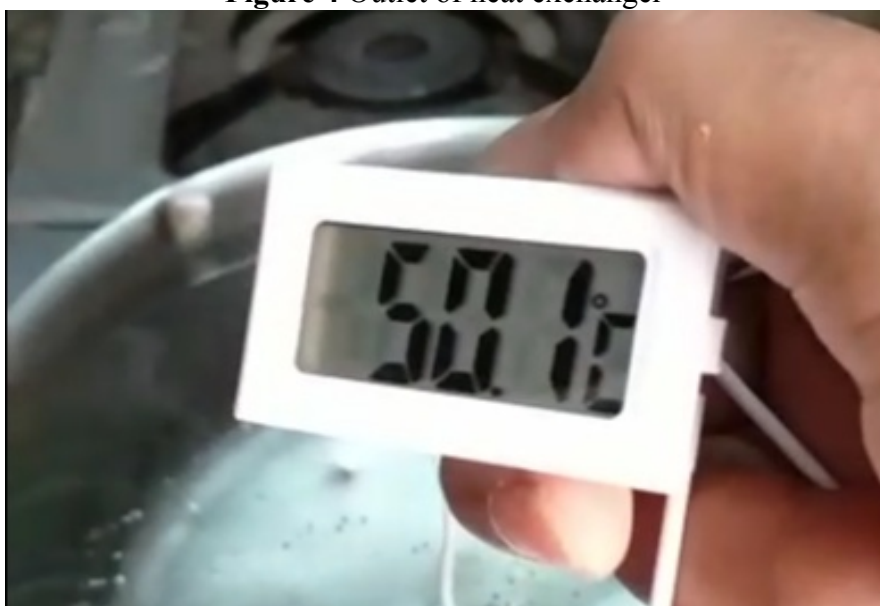
Figure 5 Measuring water temperature by using Thermocouple
