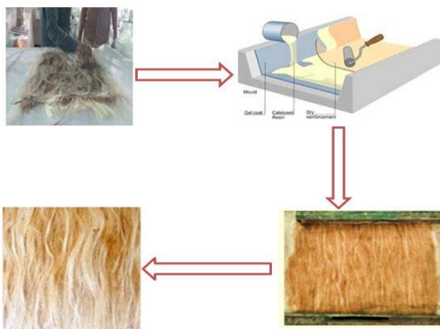
Figure 3 Hand-lay up technique for fabrication of composite.
