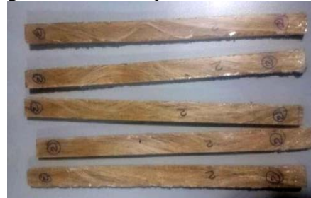
Figure 6 Tensile test specimens of sisal reinforced polyester composite.
