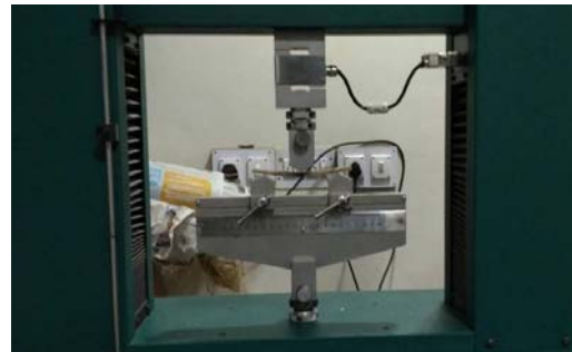
Figure 5 UTM setup for flexural testing.
