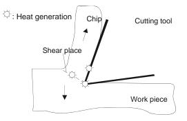
Figure1: Generation of heat during turning of metal [8]
