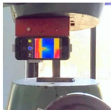
Fig. 3 Thermal Camera Setup on UTM
