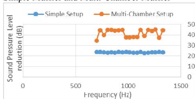
Fig. 7: Comparison of Numerical Simulation values of Simple Muffler and Multi-Chamber Muffler
