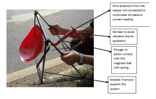
Efficiency: The obtained Model undergone several iteration as explained above to increase the output required. The current generated as per the Multimeter reading is 0.2-0.45V. This can be increased by further refining the model such as increase in the number of turns in the coil, oscillation of Magnetic ball inside the coiled cylinder, etc. The surface area required is feasible due to its compatibility. The generated current can be stored in the battery and then it is utilized.
