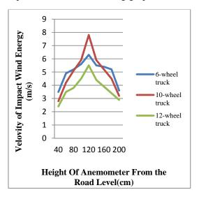
Analysis carried on the side of the divider of highway for different vehicles as shown in the figure:
