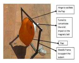
Stage 3: Development of flow path for magnetic ball followed by actuation system
