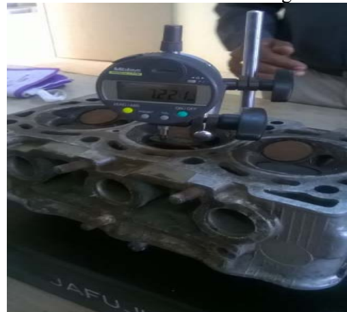
Fig 12: Experimentation of Valve displacement
