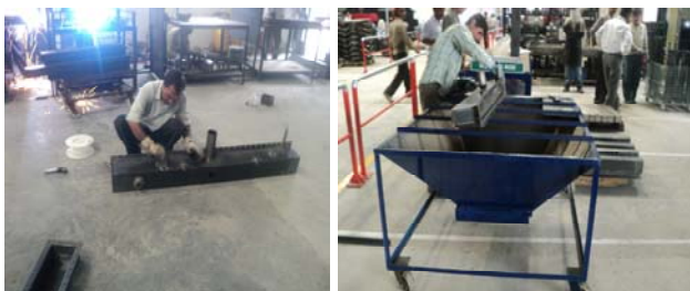
Figure 3: Right thing is in right place Spatter removing after welding
