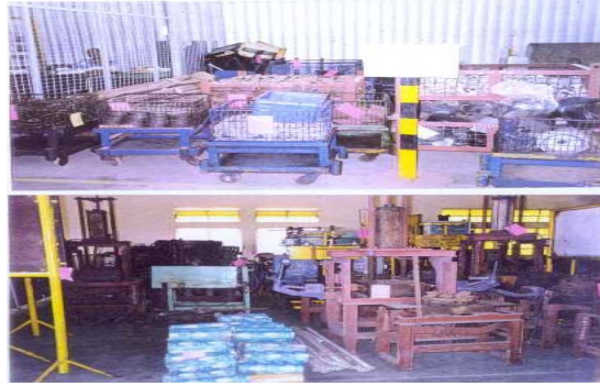
Figure 1: Improper arrangement of the parts (Jigs / Tooling)mm
