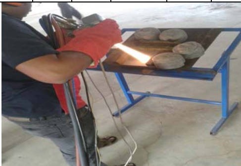
Fig.6 HVOF Spraying Process
