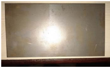
Fig.2 Mild Steel substrate
