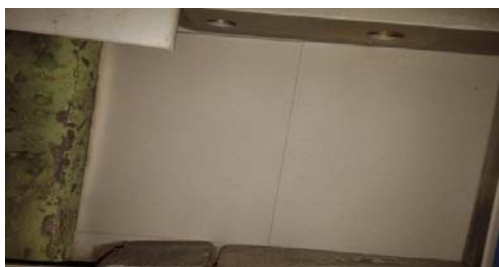
Fig.7 HVOF Coated Sample
