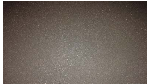
Fig.4 Grit blasted sample surface
