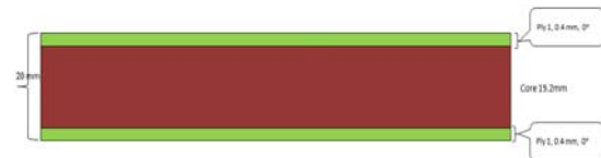
Fig.7 Material Properties of composite sandwich panel –Mono core
