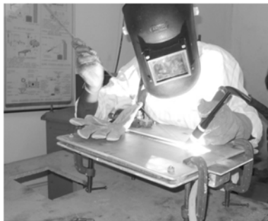
Fig.2 Welding of Ti-6Al-4V sheets
