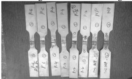
Fig.5 Tensile specimens of Ti-6Al-4V
