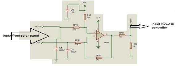
FIG.3: Shunt resistor in series to solar panel
