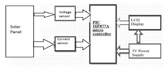
Fig. 1. Block diagram of solar energy measurement system
