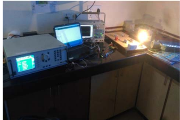
Fig. 6 Complete setup of TCSC hardware
