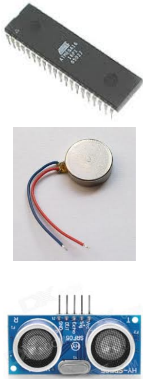
Fig.3.2 AVR, Vibration Motor, Ultrasonic Srf05 Sensor.
