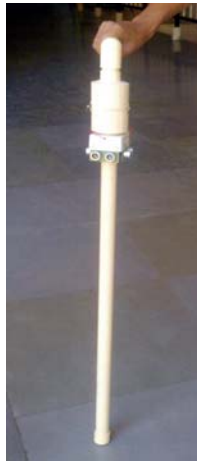
Fig.3.1 Prototype Design of Ultrasonic Smart Cane
