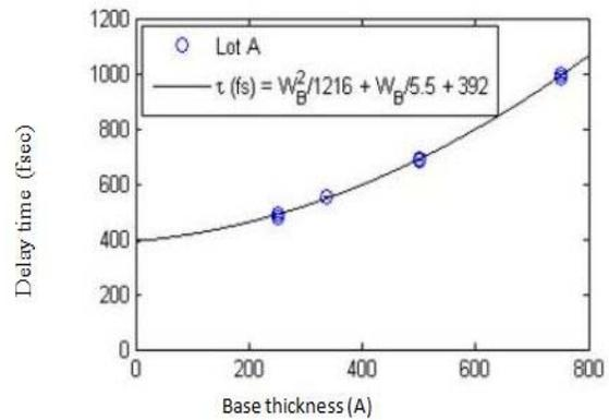
Fig. 9 Delay time  $\tau_T$  versus base thickness  $W_B$  [26].
