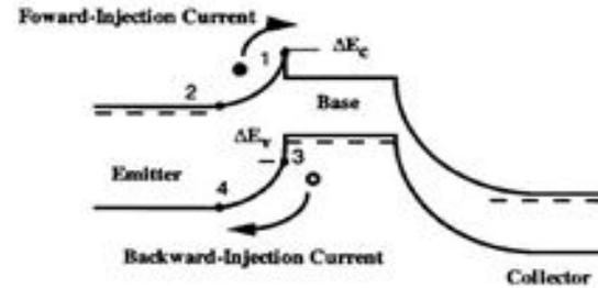
Fig. 2 Band diagram of NPN HBT under normal forward active mode.
