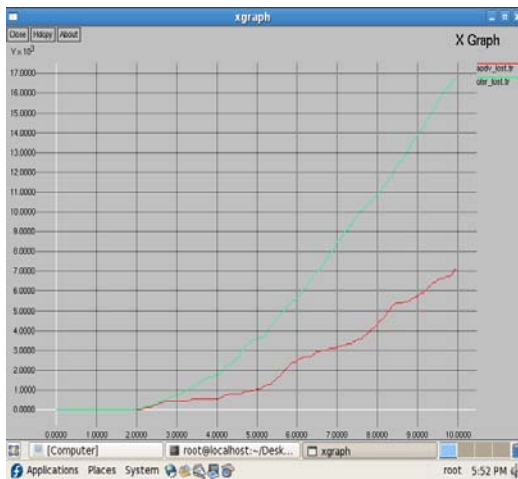
Fig 10: Comparing lost packets of AODV and OLSR
