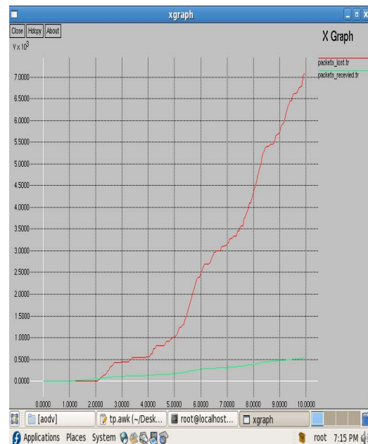
Fig 2: AODV graph comparing packets lost and packets received
